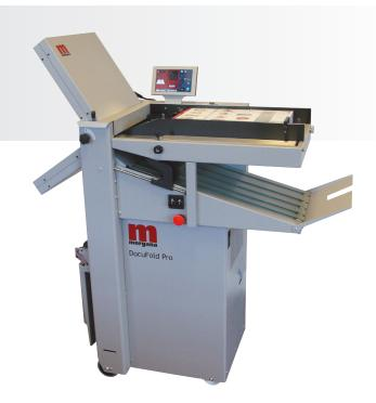
the fly if the fold plates or delivery roller needs to be moved. Within this SmartScreen panel are a counter and batching facility which are standard features. A further feature of the sophisticated SmartScreen is the ability to memorise and store repeated jobs in the alpha numeric memory which can then be retrieved within seconds.
